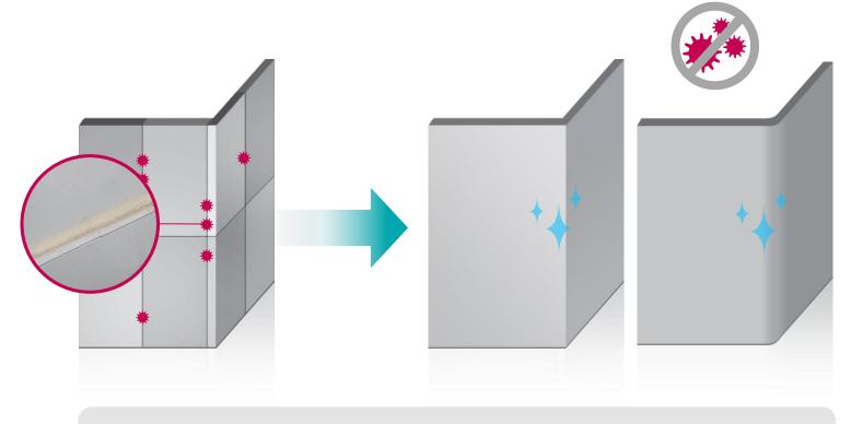
**Seamless joints** between two panels, a smooth and non-completion which does not grip dust
