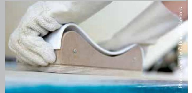
HI-MACS® boasts a simple heating process and three dimensional thermoforming capabilities. This enables greater forming flexibility compared with other conventional materials so that spectacular ideas can quickly take on a concrete shape. HI-MACS® Ultra-Thermoforming formula allows the material to be
