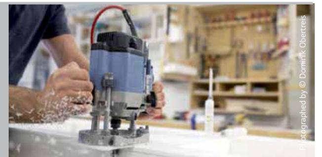
Although HI-MACS® is almost as robust as stone, it can be worked in the same way as wood. Using conventional carpenters' tools, this solid surface material can be sawn, routed or drilled. It lends itself to the creation of an endless variety of multi-dimensional forms and much, much more.
