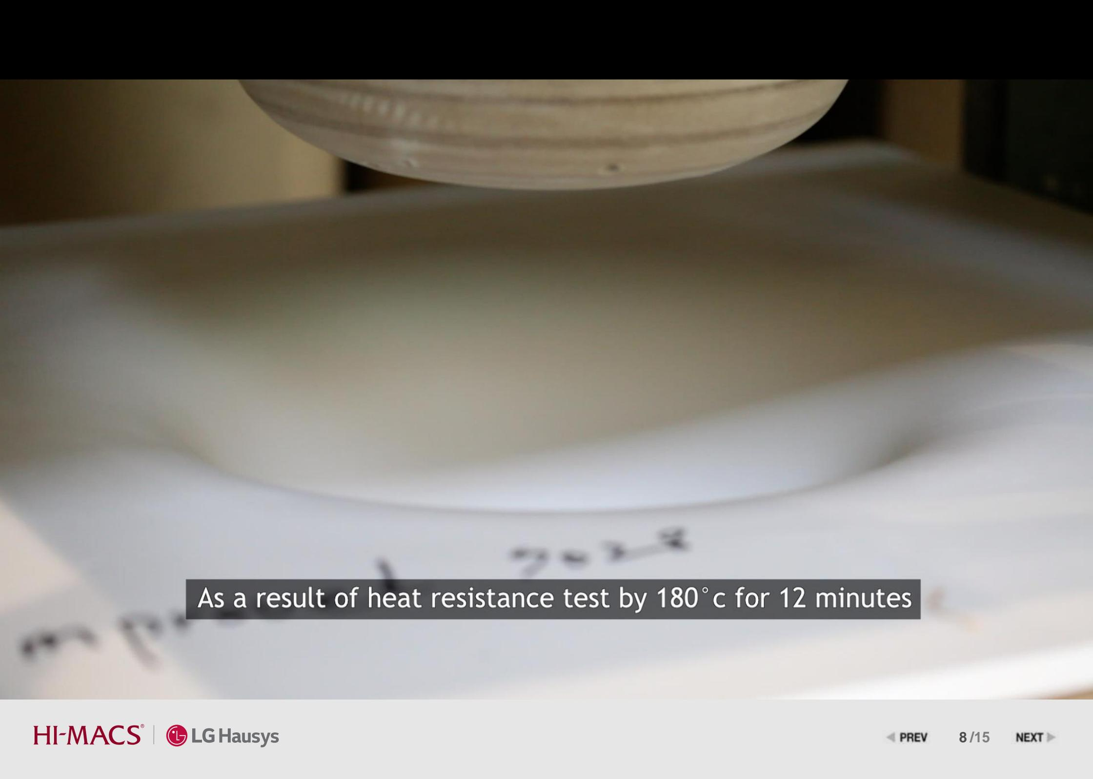
As a result of heat resistance test by 180°c for 12 minutes
