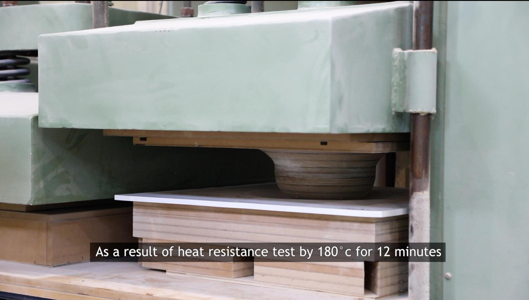
As a result of heat resistance test by 180°c for 12 minutes
